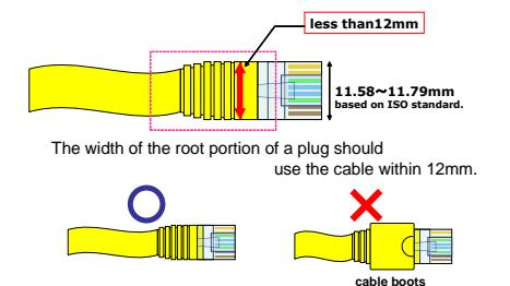
Refer to the left figure which does not get used to use for the cable with boots (with a connector cover).
