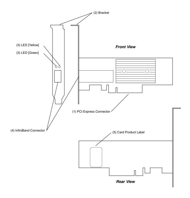
(1) PCI Express connector Connect with PCI slot in the server.
